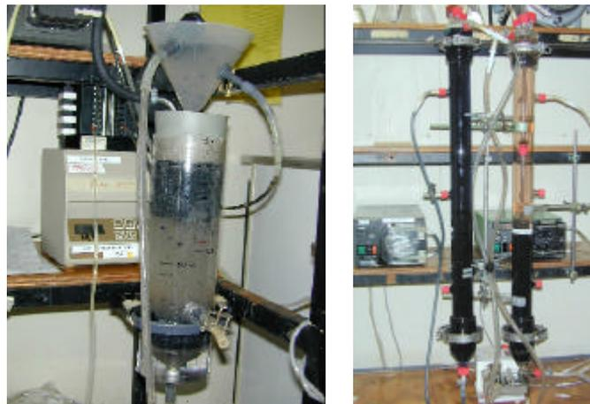
*Bioreactors used for anaerobic tests: UASB (left). EGSB (right).*
