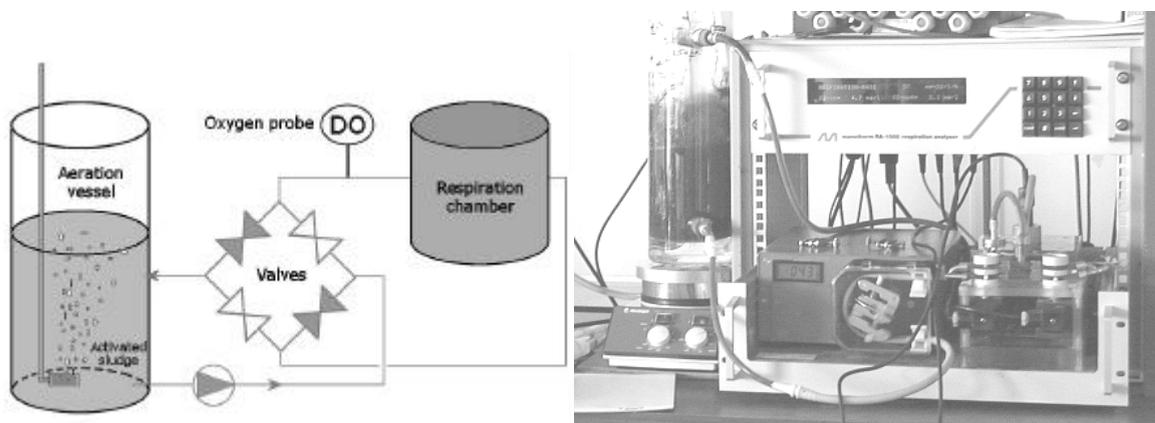
*Schematic representation and photo of the used respirometer*
